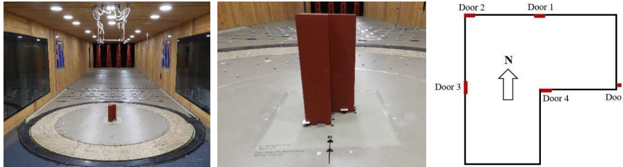
Figure 3. Wind-tunnel study model and door location
